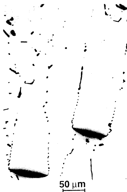
Fig. 4. Photomicrograph of lenticular and elongated voids in oxide fuel migrating under the influence of temperature gradient roughly normal to the major pore dimension (after Sens [14]).
